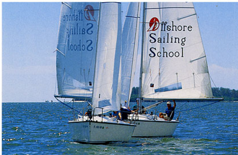
Figure 8-4. Overtaking rule: boat behind is overtaking and has to give way.
